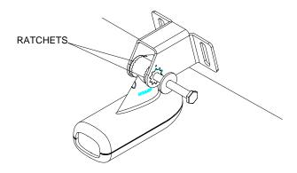
3. Once you determine the correct position for the ratchets, assemble the transducer as shown at left. Don't tighten the lock nut at this time.
